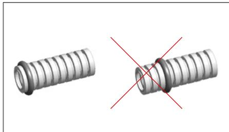
3. Please insert the clip for the actual corrugated pipe connector (or adapter for the smooth hose) into the next groove behind the seal and place it around the corrugated pipe. Then slide the hose into the connector and lock it in place. Note: the corrugated pipe must encounter a slight resistance when being inserted. If there is too little or too great a resistance during insertion, the wrong seal has been selected.
